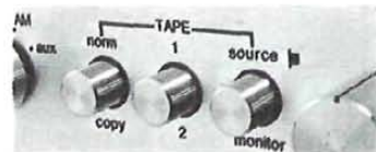
Two completely independent tape monitors.
